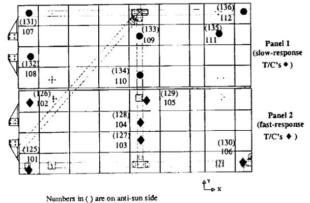
Fig. 4. Typical Solar-Panel Thermocouples
