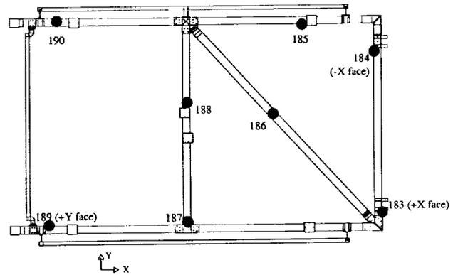
Fig. 5. Typical Panel Support Structure (PSS) Thermocouples
